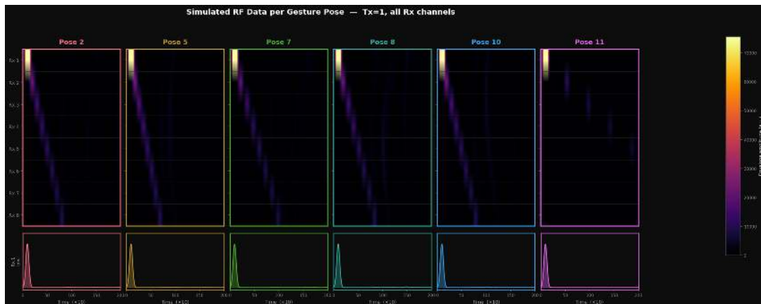
Figure 4: Hilbert envelopes per receive channel for a single transmitter firing on the linear array. All six poses of Subject 1.
